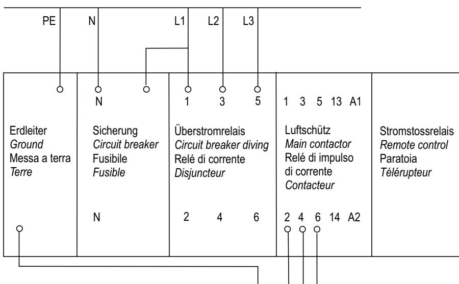
Pumpenaggregat / Towards engine / Gruppo pompa / Branchement de moteur
